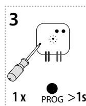
Press of programming button on actuator RFDEL-71B shorter than 1 second will finish programming mode, LED switches off.
