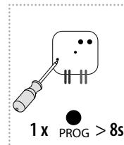
By pressing the programming button on the actuator for 8 seconds, deletion occurs of the actuator's entire memory. The LED flashes three times and goes out, then again flashes three times and goes out.
