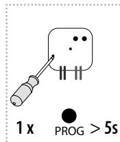
By pressing the programming button on the actuator for 5 seconds, deletion of one transmitter activates. The LED flashes in an interval of 1s.
