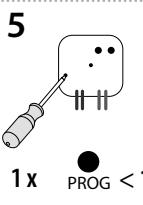
Press of programming button on actuator RFDEL-71B shorter than 1 second will finish programming mode, LED switches off.
