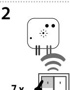
Seven presses of your selected button on the RF transmitter assigns the function ON/OFF (must be a lapse of 1s between individual presses).
