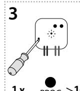
Press of programming button on actuator RFDEL-71B shorter than 1 second will finish programming mode, LED switches off.
