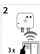
Three presses of your selected button on the RF transmitter assigns the function light scene 3 (must be a lapse of 1s between individual presses).
