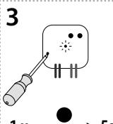
Press of programming button longer than 5 seconds, will activate actuator into timing mode. LED flashes 2x in each 1s interval. After releasing the button, the time of the sunset function begins to count down (period of complete dimming of the light).
